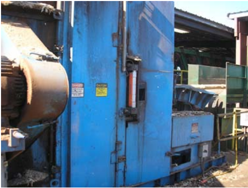
Type MD Log Scanner mounted directly on Brunette debarker at Goshen Forest Products, in Goshen OR,
